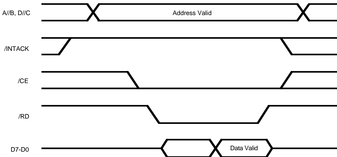
Figure 2-5. Z85X30 Read Cycle Timing
