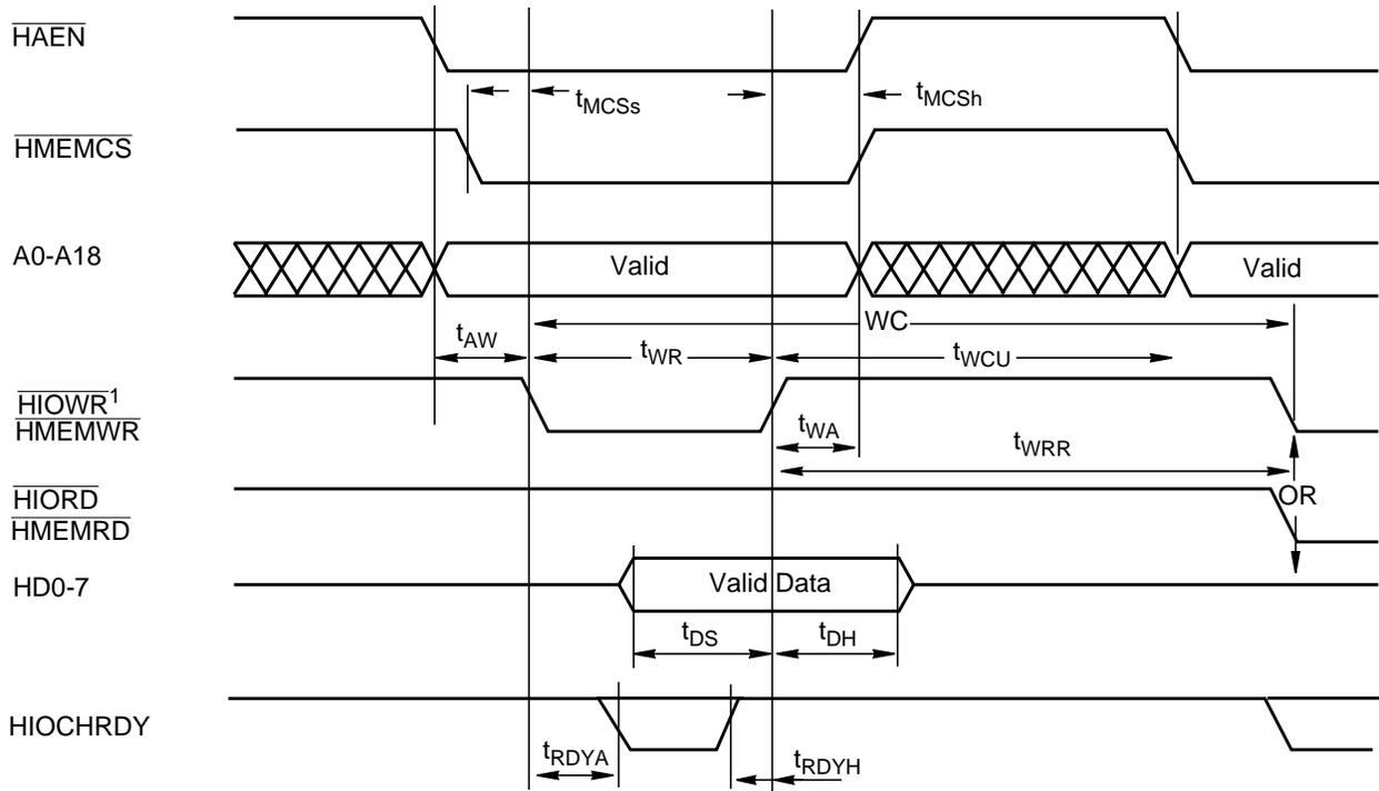
Notes: 1. Either HIOWR or HMEMWR is active, for access to I/O devices or the shared memory, respectively.
