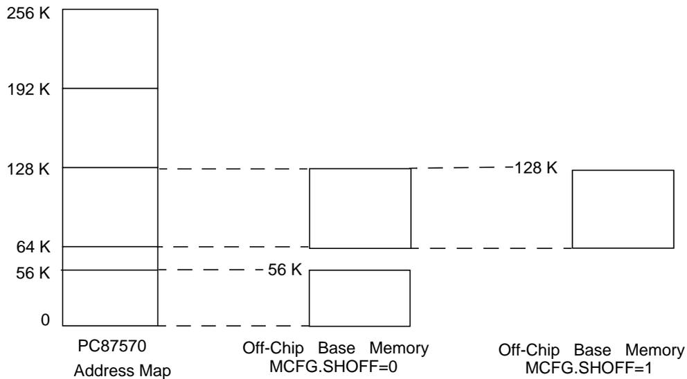
Figure 2-3. Off-Chip Base Memory (Zone 1) Address Range
