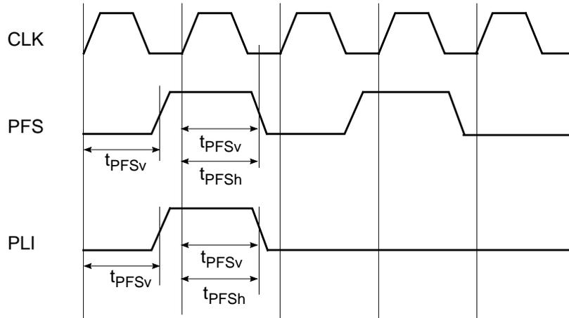
Figure 19-23. Pipe Status Signal (PFS and PLI) Timing
