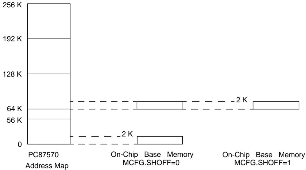
Figure 2-2. On-Chip Base Memory (Zone 1) Address Range
