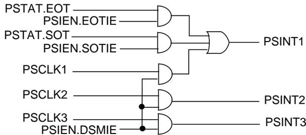
Figure 12-2. PS/2 Interface Interrupt Signals
