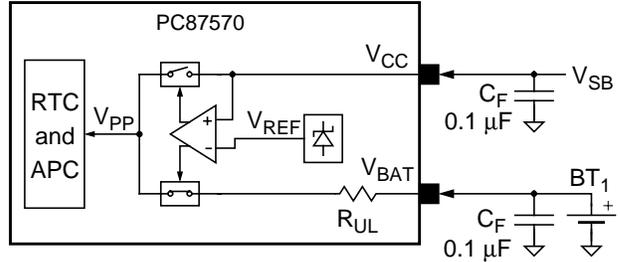
1. Place a 0.1  $\mu\text{F}$  capacitor on *each*  $V_{CC}$  power supply pin as close as possible to the pin, and also on  $V_{BAT}$ .
