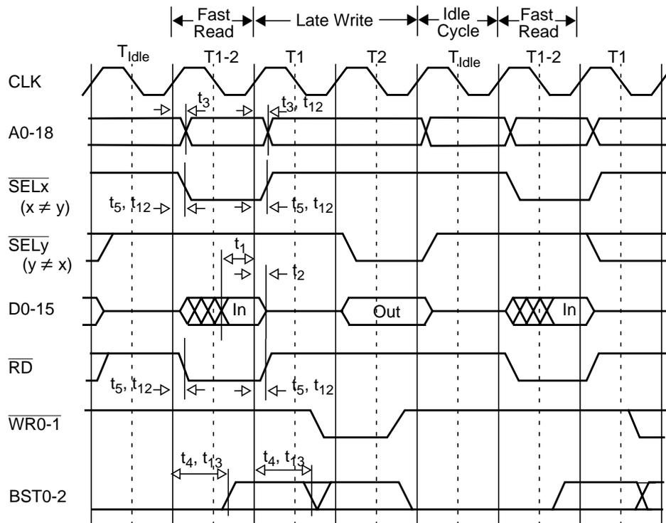
Figure 19-12. Fast Read Bus Cycle, AC Timing
