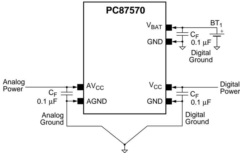
1. Place a 0.1 μF capacitor on *each* V<sub>CC</sub> power supply pin as close as possible to the pin, and also on V<sub>BAT</sub>.
