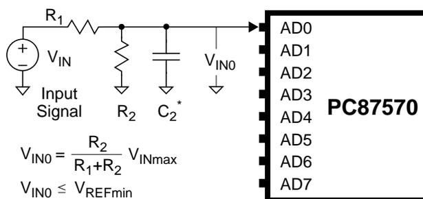
$$V_{IN0} = \frac{R_2}{R_1 + R_2} V_{INmax}$$
