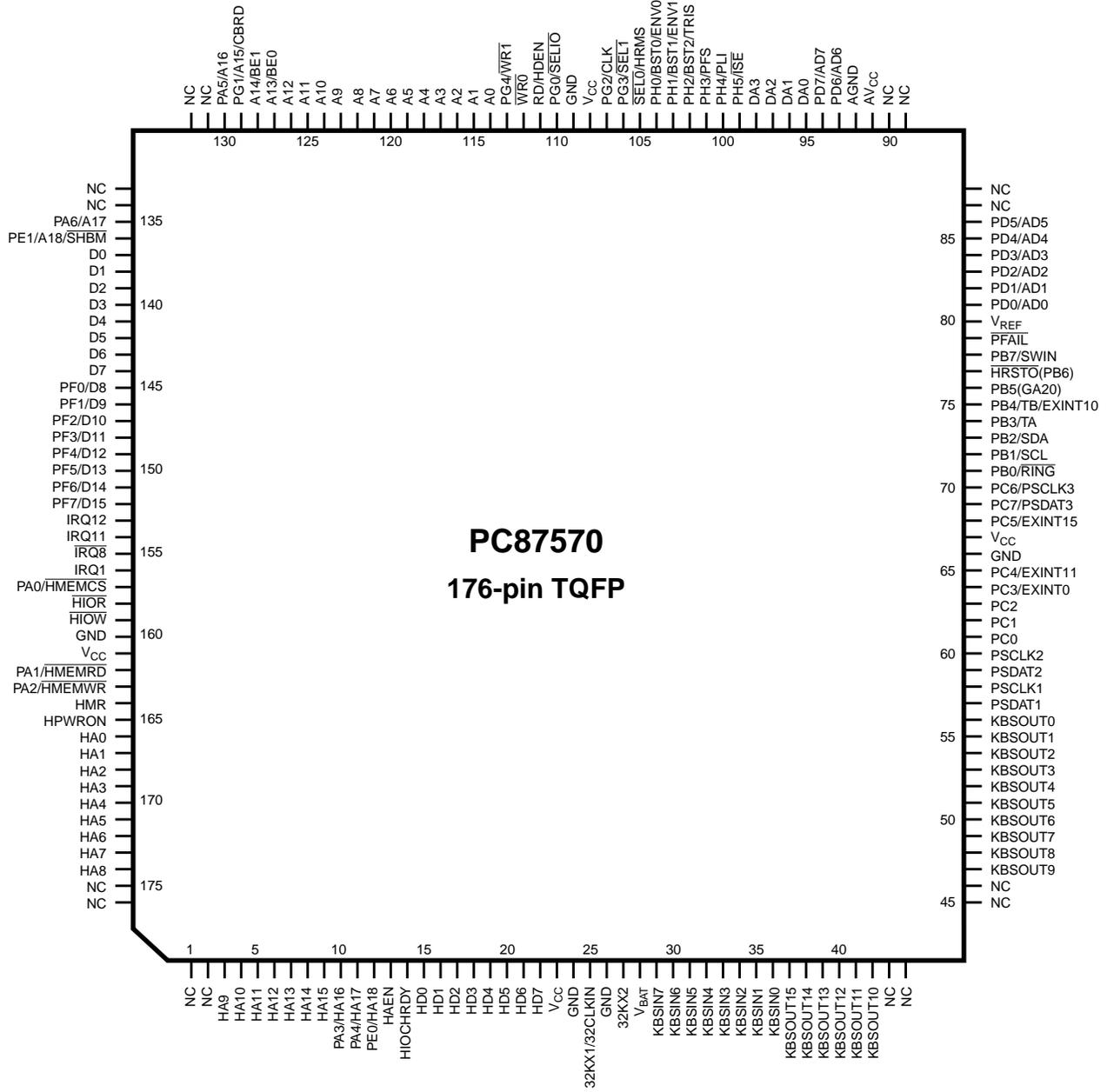
**176-pin Thin Quad Flatpack (TQFP)**
