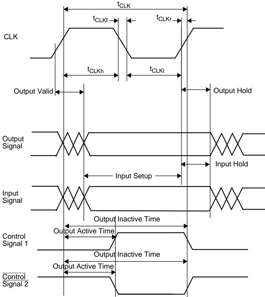
Figure 19-6. Clock Waveforms
