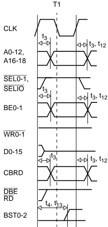
Figure 19-13. Core Bus Monitoring Bus Cycle, AC Timing
