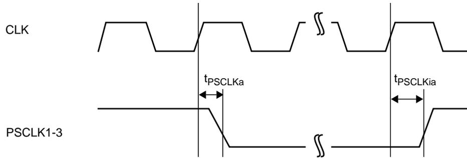
Figure 19-30. PS/2 Clock Signal Pulled Low by PC87570
