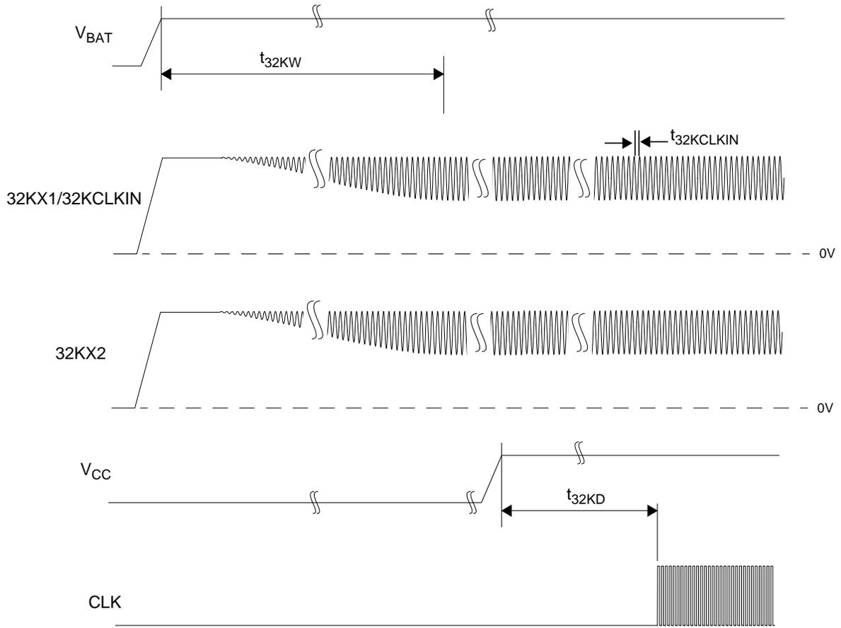
Figure 19-5. 32K Waveforms
