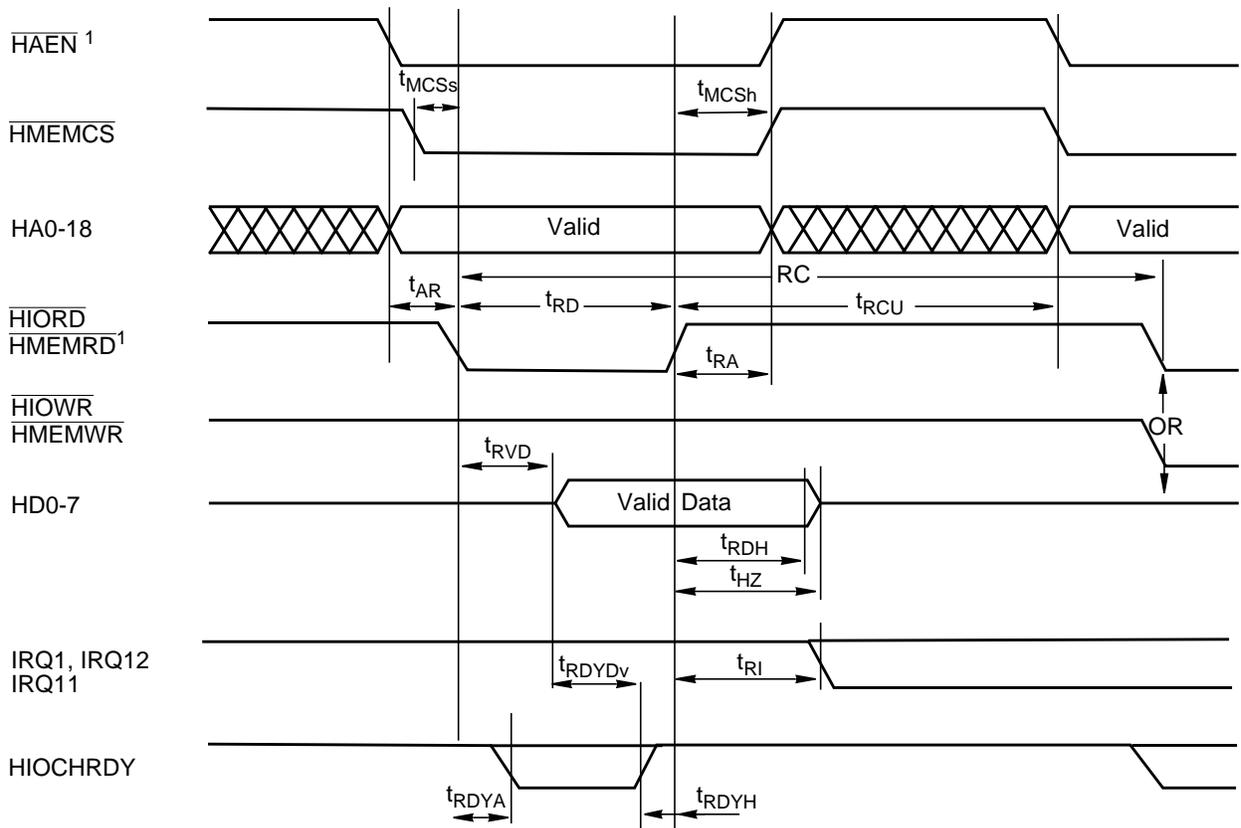
1. Either  $\overline{\text{HIOR}}$  or  $\overline{\text{HMEMRD}}$  is active, for access to I/O devices or the shared memory, respectively.
