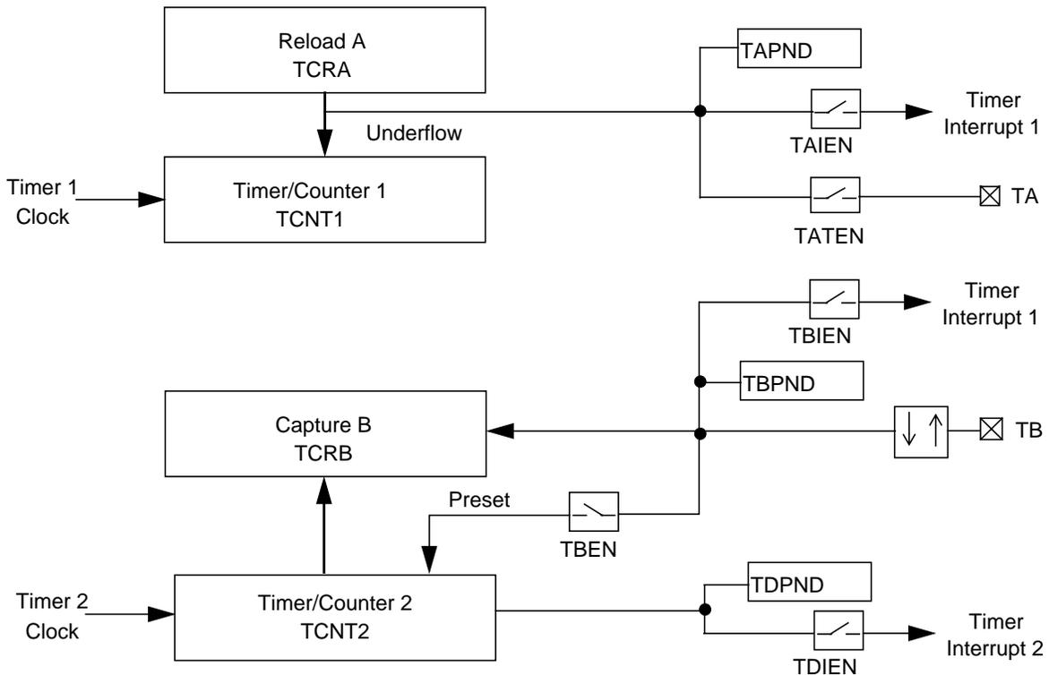
**Figure 14-7. Mode 4, Input Capture and Timer**
